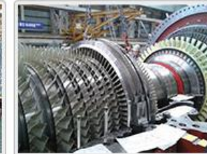
Blade Ring Assembly & Clearance Check
